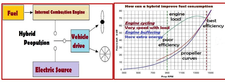
Propulsion using a fueled power source (diesel engine) or through a stored energy source (battery bank and electric motor)
